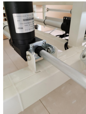
Operating bed by manually turning the crank before cut the power supply
