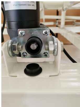
Operating bed by manually turning the crank before cut the power supply
